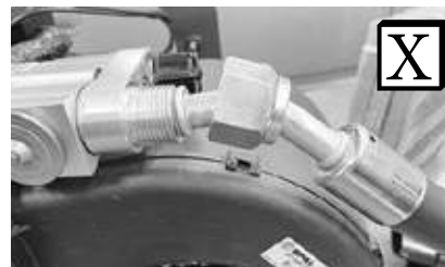
Improperly Seated O-ring Land
