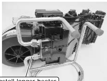
Install longer heater hardline onto evaporator module lower connection
