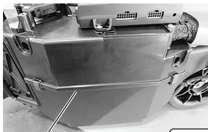
Route main wiring harness (white/yellow/purple) through 7/8" wiring grommet on kick panel
