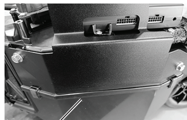
Route red, white and blue wires from main harness through 7/8" wiring grommet on kick panel
