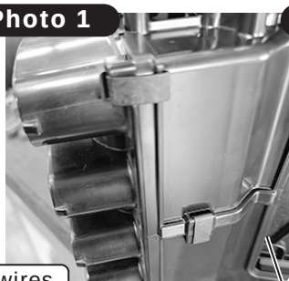
Route heavy gauge orange and white wires through 7/8" wiring grommet on kick panel
