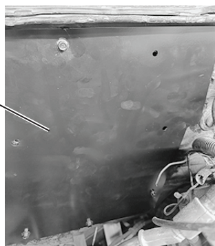
Temporarily install firewall cover and drill remaining holes with 5/16" drillbit
