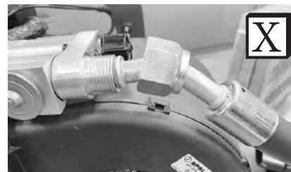
Improperly Seated O-ring Land
